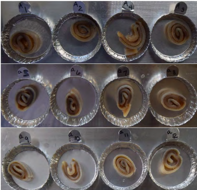
Figure 8. Remains of samples from the 10-mm slices of Item C, Collagen, after 6, 8 and 24 hours (from top to bottom) in digestive fluids.
